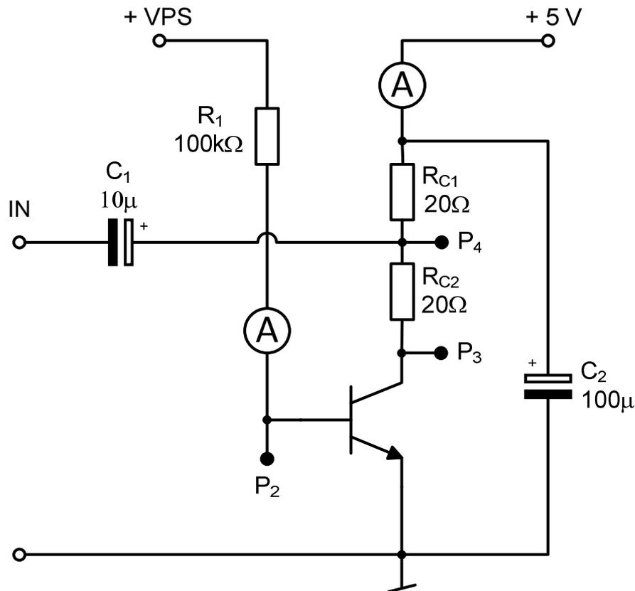
Fig. 2. A circuit used for determination of the output conductance of BJT ( $h_{22e}$ ).
