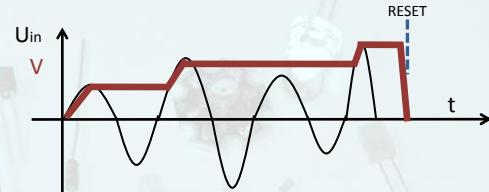
By means of peak detector DC voltmeter can measure amplitude of variable waveforms.
