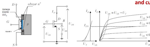
**depletion P-channel:**  $U_{DS} < 0$ ,  $I_D < 0$ ,  $U_{GS} > 0$  i  $U_P > 0$
