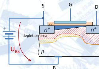
$$V_T = V_{T0} + \gamma (\sqrt{\varphi_s - U_{BS}} - \sqrt{\varphi_s}) \quad \text{for NMOS}$$
