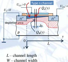
One has to integrate the equation (1) „along the channel length”, from 0V to  $U_{DS}$ :
