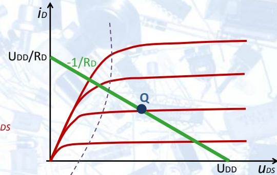
$$i_D = \frac{W}{L} \mu C_{ox} \left( u_{GS} - V_T - \frac{u_{DS}}{2} \right) u_{DS}$$
