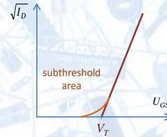
Diffusion mechanism of current flow
