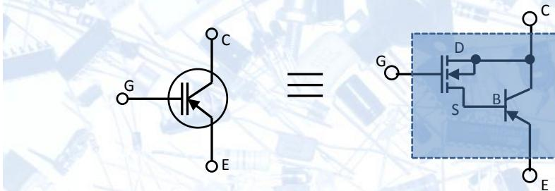
IGBT transistor combines the positive characteristics of the MOSFETs
