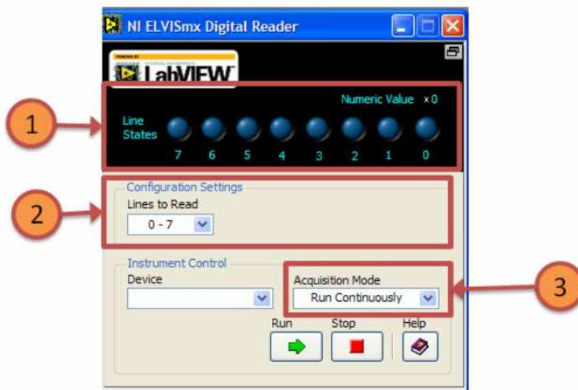
Fig. 11. DigIn SFP with important controls labeled
