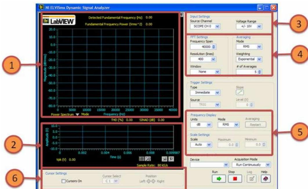
Fig. 9. DSA SFP with important controls labeled
